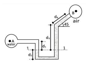
**Question 4**: Taking into consideration the manometer system shown below find the absolute pressure at point A. ( $p_{\text{atm}}$ =101.34 kN/m<sup>2</sup>,  $\gamma_{\text{glycerin}}$ =12.36 kN/m<sup>3</sup>,  $\gamma_{\text{water}}$ =9.81kN/m<sup>3</sup>)
