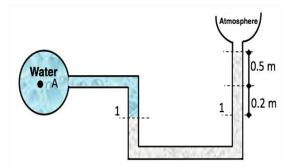
**Question 2**: in the manometer system given below, the absolute pressure of the enclosed gas is  $P_{gaz} = 39.24 \text{ kN/m}^2$ . Find the horizontal distance X. ( $\gamma_{yag} = 7.85 \text{ kN/m}^3$ ).
