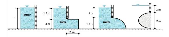
**Question 2:** Schematize the horizontal and vertical pressure forces acting on the surfaces ABCD. (Width perpendicular to the figure plane is 1m).
