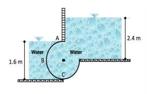
Question 8: The width of the semi – cylindrical gate ABC (perpendicular to the figure plane) shown in the figure is 5 m. One side of the gate is pressurized air. Find the horizontal and vertical components of the force acting upon the gate. Answer: Fhorizontal=195.20 kN, Fvertical=308.23 kN
