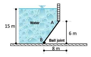
**Question 6:** Taking the width of the cylindrical gate perpendicular to figure plane as 1 m, find the horizontal and vertical components of the force and magnitude of the resultant force acting upon the gate and the coordinates of application point with respect to point A.
