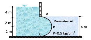
**Question 9**: Find the pressure force acting on the cylindrical gate for the given chamber system. For the state of equilibrium, calculate the height  $h_2$  in terms of the other parameters.
