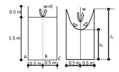
**Answer 3:** a)  $\omega_{\text{max}} = 8.86 \text{ rad s}^{-1}$ ; b)  $\omega = 15.34 \text{ rad s}^{-1}$ ;  $p_{eksen} = 1.27 \times \gamma = 12.46 \text{ kN/m}^2$  and  $p_{cidar} = 1.73 \times \gamma_{su} = 16.97 \text{ kN/m}^2$
