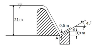
Results:  $v_a = v_b = 20 \, m/s$  ;  $q = 12 \, m^3/s \, / m$  b-  $R = 186.78 \, kN$
