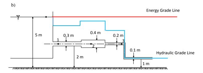
**Question 2:** The flow is opened to the atmosphere at point D which is fed by a very wide reservoir that has a water surface elevation of 5 meters as shown in the figure given below. Elevation of the horizontal axis BC is 1 meter. At sections AB and CD the diameter of the pipe is 0.2 meters. The flow is ideal (inviscid) and absolute atmosphere pressure is 9.81 N/cm<sup>2</sup>.
