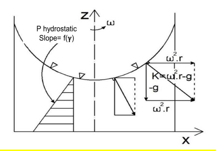
For a fluid of unit mass, the change in pressure with distance in a certain direction is equal to the specific weight of the body.
