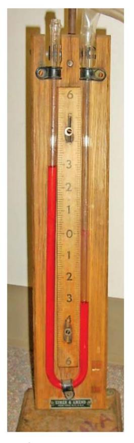
A simple U-tube manometer, with high pressure applied to the right side.
