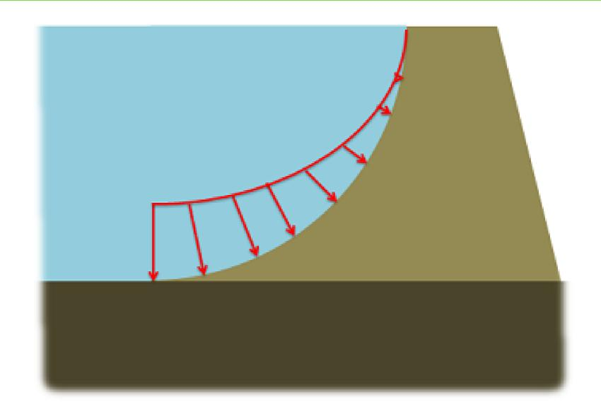
In this case, however, the elemental forces are not parallel to each other. As a result, the total pressure force cannot be calculated directly. It is rather calculated with the help of components.
