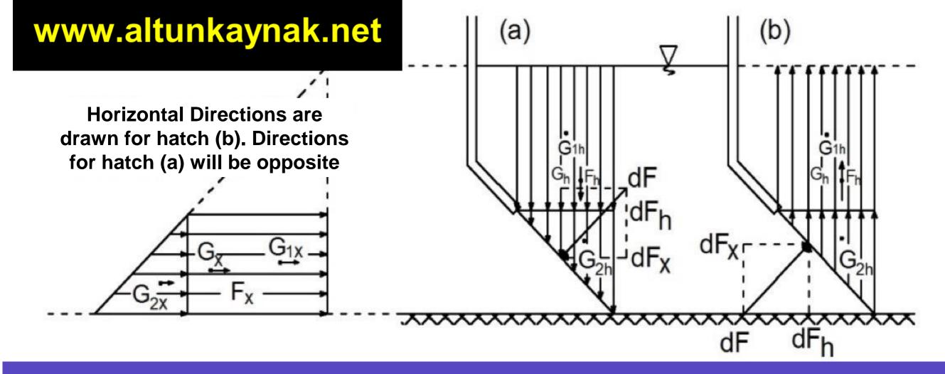
2. When determining the points at which Fx and Fh are acting, one should take in to consideration the center of gravities of the areas used in the calculation of the forces.
