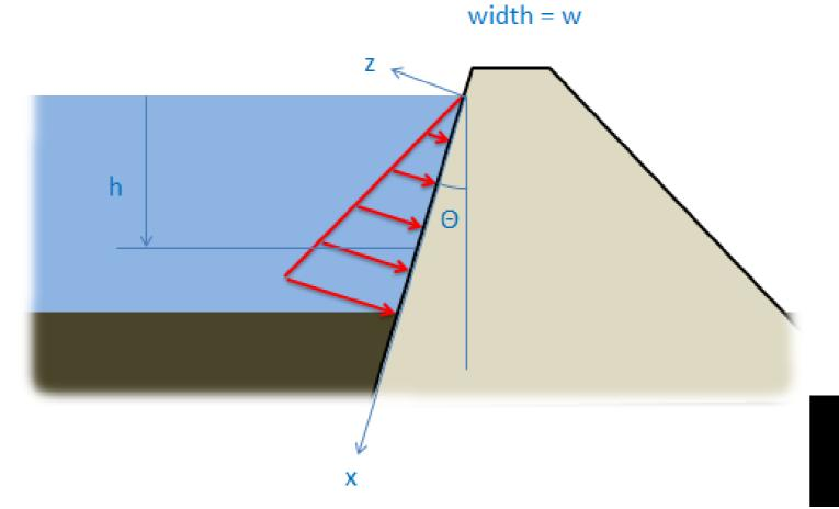
In this case, the elemental pressure forces are parallel to each other. As a result, the resultant force can be calculated directly.
