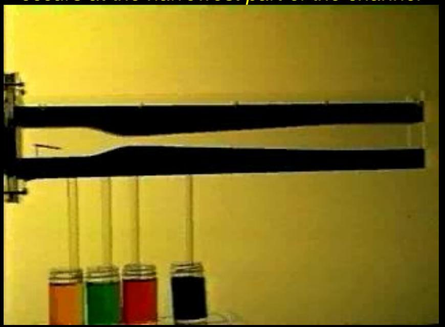
The same principle is used in a garden sprayer so that liquid chemicals can be sucked from the bottle and mixed with water in the hose.
