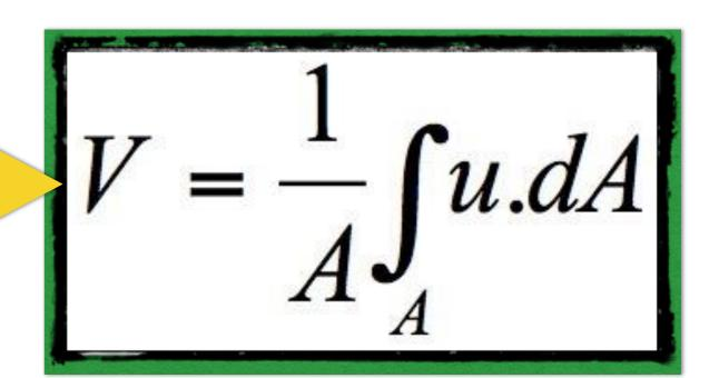
It is the velocity which is used to determine the discharge, Q, when multiplied by the cross-sectional area, A, of the channel.
