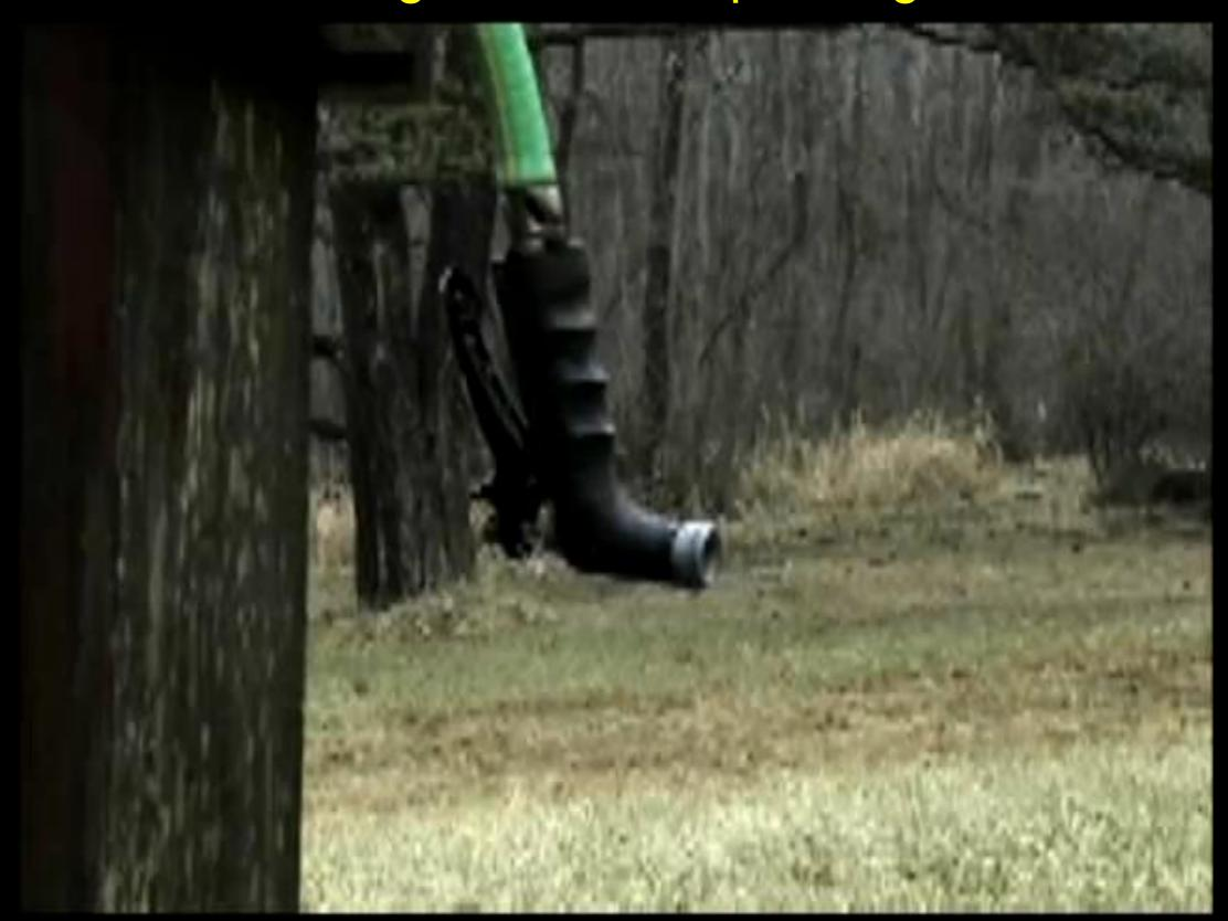
Work must be done on the device shown to turn it over because the system gains potential energy as the heavy (dark) liquid is raised above the light (clear) liquid. This potential energy is converted into kinetic energy
