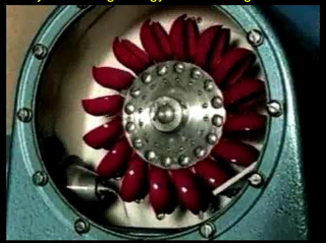
Energy of the water is converted into the output energy of the turbine
