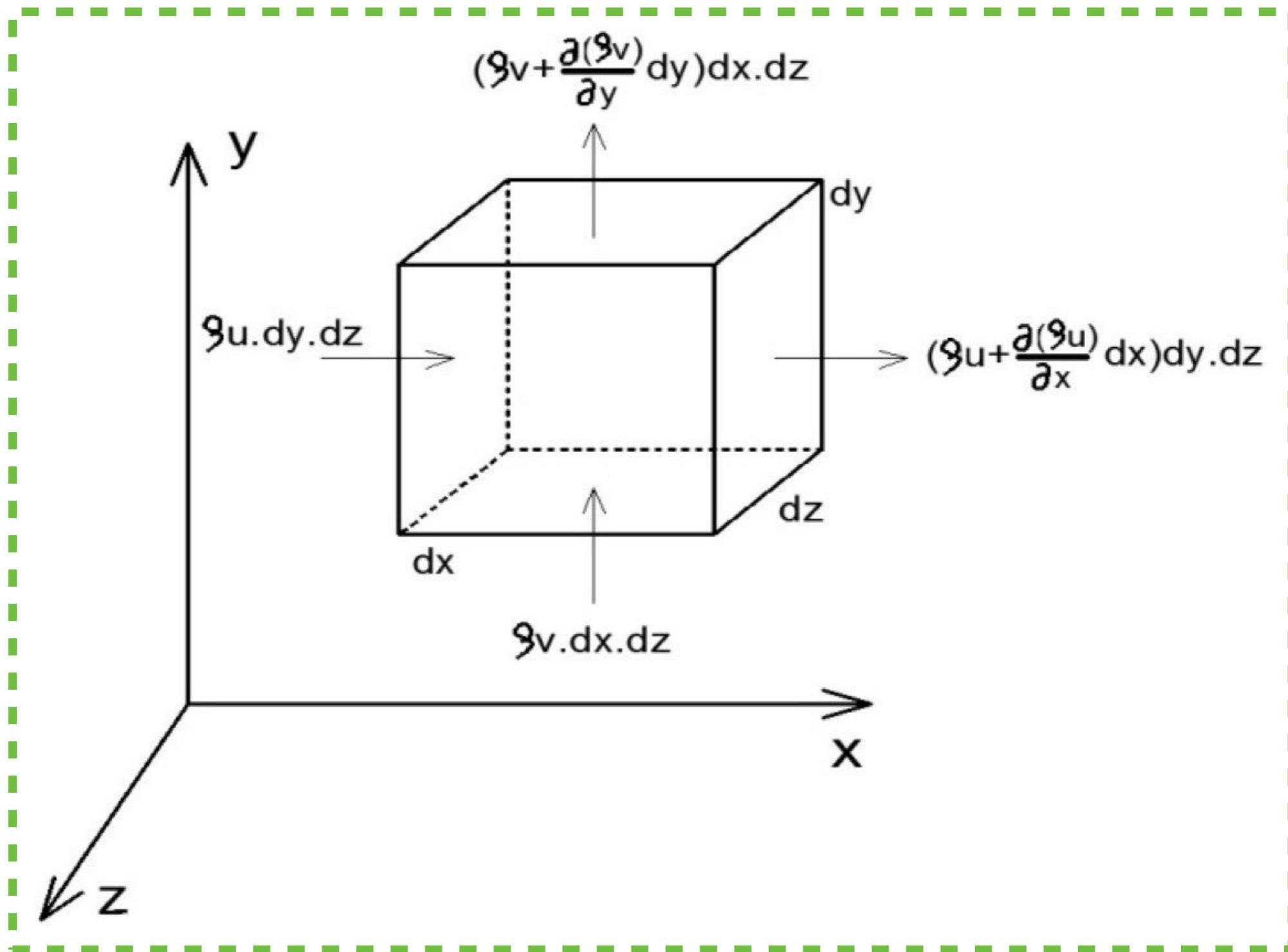
The same principle can be used to determine the mass flow rate on the other plane
