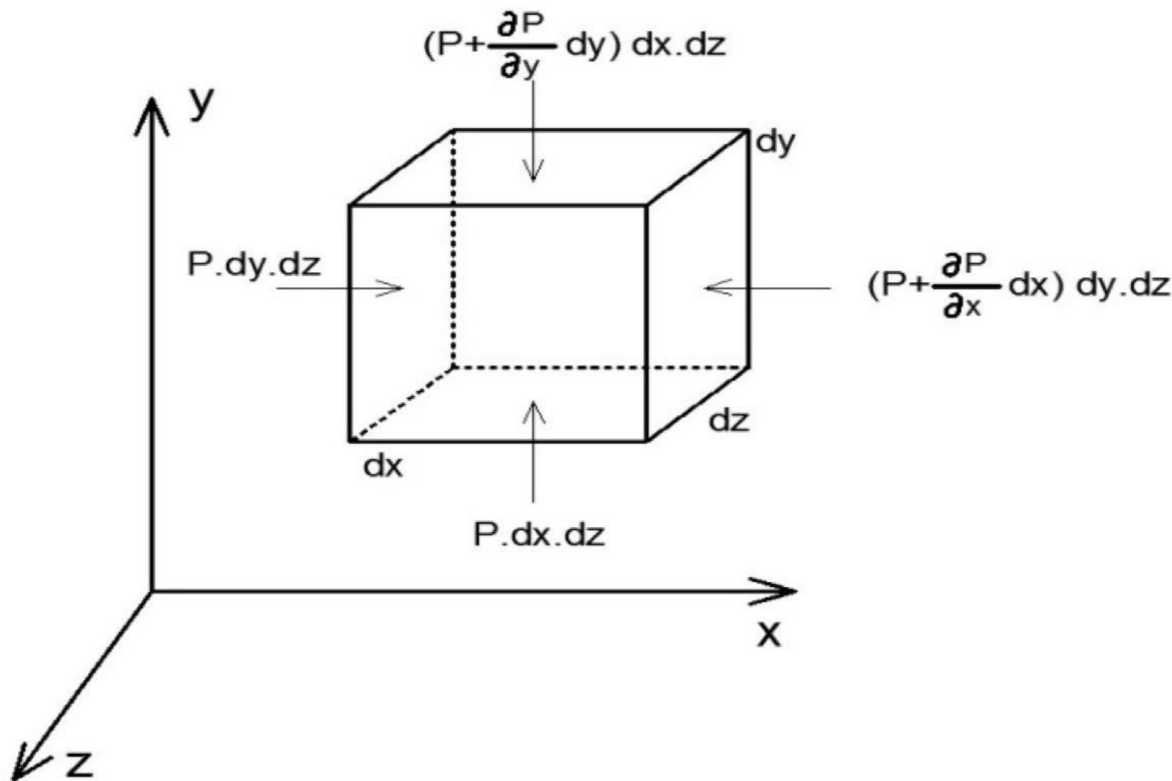
Let the components of the volumetric force (weight) of a unit mass be X, Y and Z, acting in the x, y and z directions, respectively
