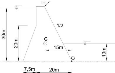
Question 15. The width of the gate in Figure is 3 m. What should be the gas pressure to hold the gate in its position considering the water pressure force on the left side?
