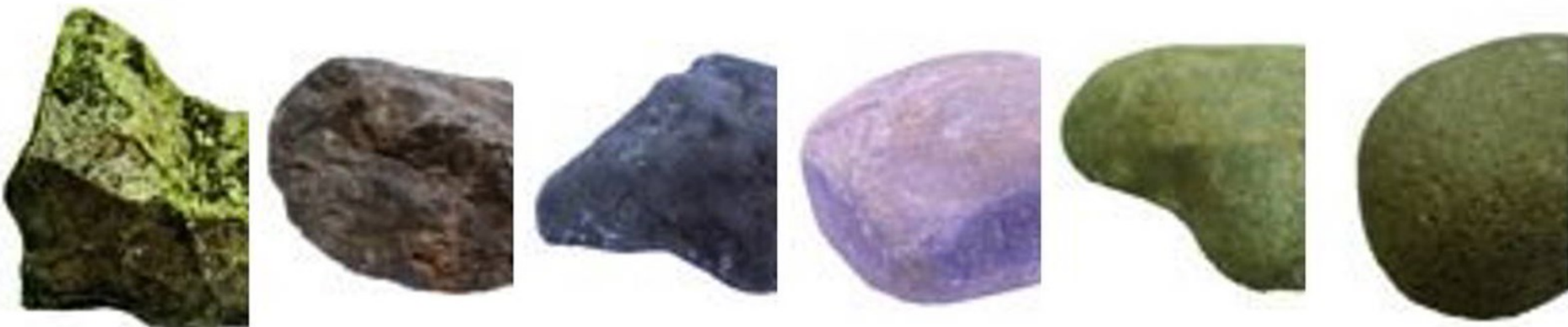
very angular angular sub-angular sub-rounded rounded very rounded For the shape expression:
